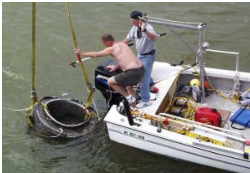
JOE GERKY, a Johnson Space Center employee (right) and Steve Van Meter, KSC robotics specialist, check the lifting slings on the thrust reverser.
