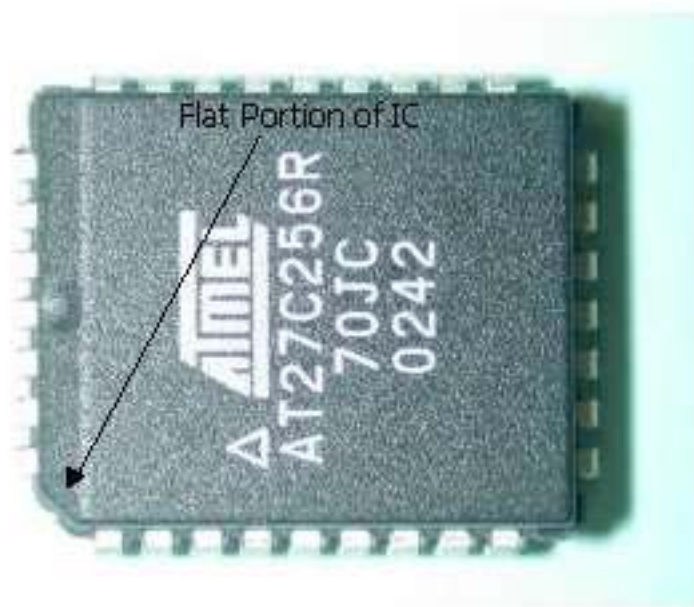
Figure 5.10.1 Shows Flat Portion of IC Chip
