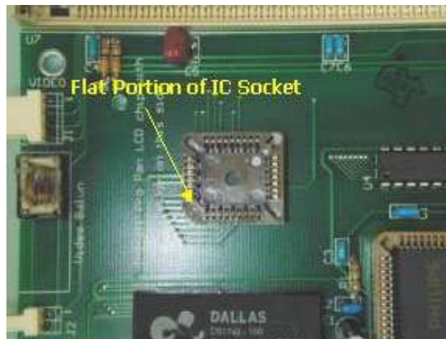
Figure 5.10 Shows Flat Corner of IC Socket
