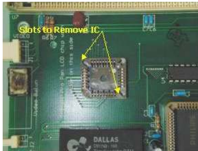
Figure 5.6.2 Shows 2 Slots to insert IC Extractor
