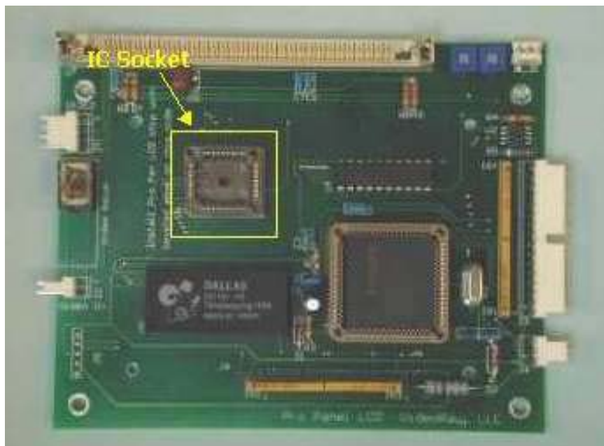
Figure 5.6 Shows the LCD Controller PCB with IC Socket
