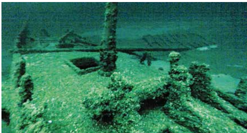
Sloop Washington mid-ship showing the log windlass, a portion of the mast, a hold, and boom lying across the deck. Photograph by Roger Pawlowski
