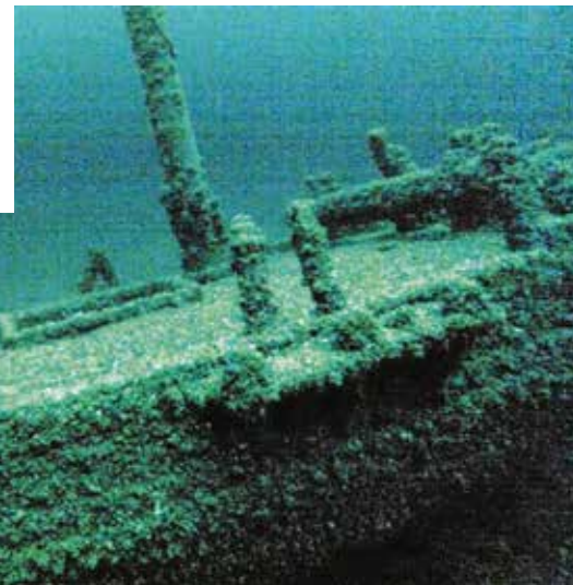
Center: Sloop Washington mid-ship showing the chain plate (lower right) log windlass, a portion of the mast, a hold, boom lying across the deck, bilge pump next to boom, and the cabin roof remains. Photograph by Roger Pawlowski
